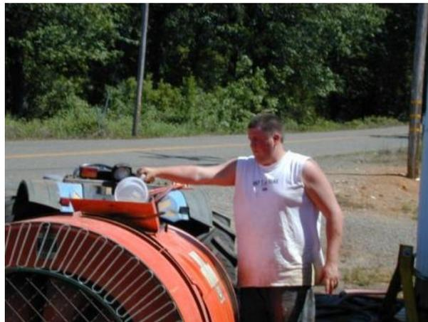
3. Measure the amount of water it takes to fill the sprayer back up to the line observed in 1.
